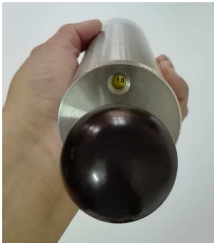
Figure E.1 – Spring hammer test apparatus
