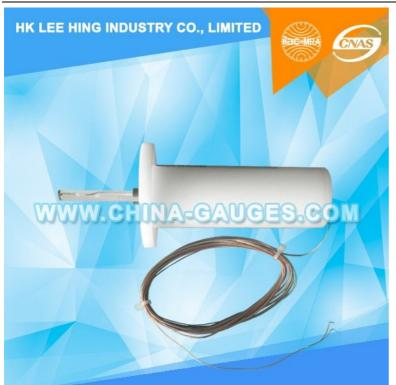
According to IEC60335-2-11:1993 fig 101 and IEC60335-2-6:1997, such as requirements preconditioning of household and similar electrical appliances drum dryers and in vertical ranges, hobs, ovens and other were surface temperature rise measurement.
