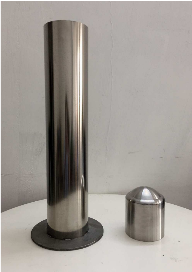
IEC60068-2-75 Figure A.3 5J Vertical Hammers for IK08 Test Ehc Striking Element.
