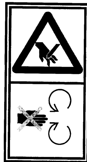
Figure E.2 — "Danger - Rotating blades. Keep hands and feet out of openings while machine is running."
