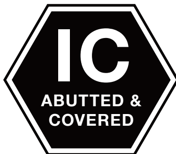
FIGURE 204 PERMITTED EXCEPTION SYMBOL FOR IC LUMINAIRES
