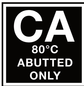
FIGURE 202 PERMITTED EXCEPTION SYMBOL FOR CA90 LUMINAIRES (FOR LUMINAIRES THAT COMPLY WITH CA80 REQUIREMENTS OF NEW ZEALAND ONLY AMENDMENT A OF AS/NZS 60598.2.2:2001)
