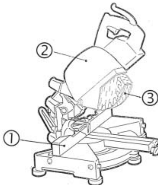
Figure Z104 - Mitre saw provided with open guard construction
