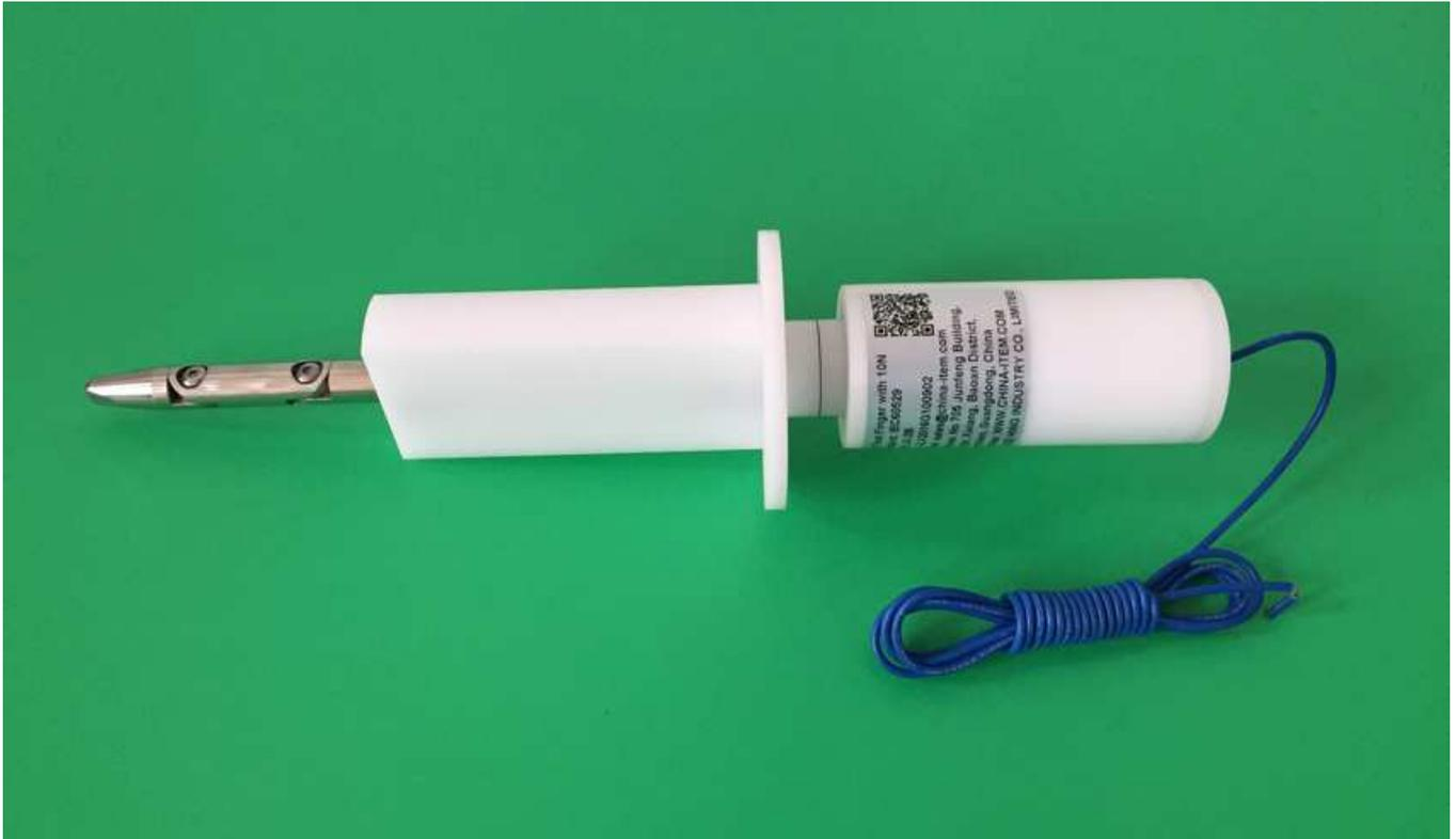
IP2X Test Probe is a precision test probe made according to Figure 1 of the IEC 60529:2013 and is used to simulate a human finger. It is also used by the standards of CSA, IRAM, UL and in most of the rules involved in the verification of accessibility to live parts.
