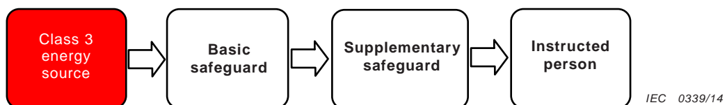
Figure 15 – Model for protection of an instructed person against a class 3 energy source
