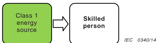
Figure 16 – Model for protection of a skilled person against a class 1 energy source
