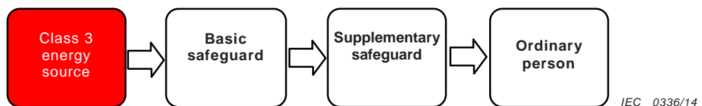
Figure 12 – Model for protection of an ordinary person against a class 3 energy source
