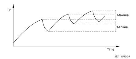
Figure B.1 – Determination of arithmetic average temperature
