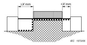
Condition: Path under consideration includes an uncemented joint with a groove on one side less than X mm wide
