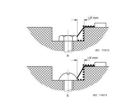
Gap between head of screw and wall of recess wide enough to be taken into account.
