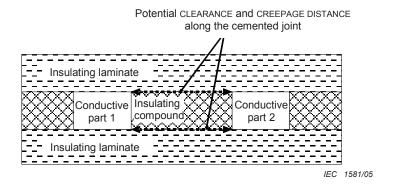
Insulating compound as SUPPLEMENTARY INSULATION or REINFORCED INSULATION
