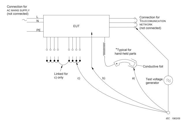
Figure 6B - Application points of test voltage
