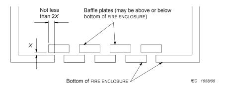
Figure 4F - Baffle plate construction
