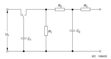
Figure N.1 – ITU-T impulse test generator circuit
