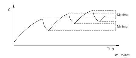
Figure C.1 – Determination of arithmetic average temperature
