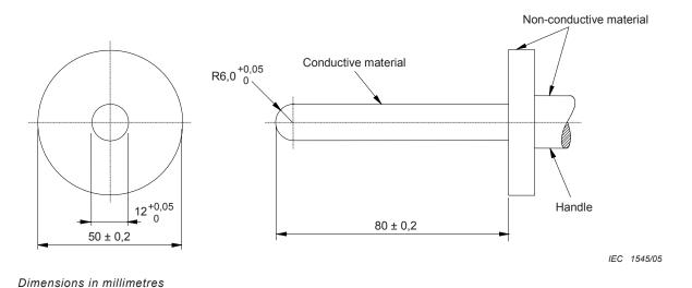
Figure 2C - Test probe
