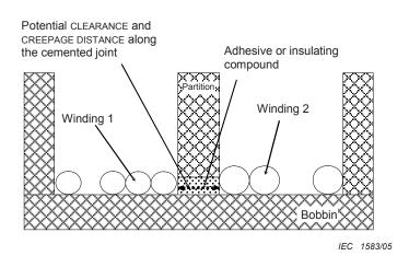
Cemented joint as SUPPLEMENTARY INSULATION or REINFORCED INSULATION
