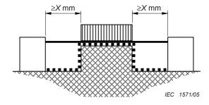
Path under consideration includes an uncemented joint with a groove equal to or more than X mm Condition:
