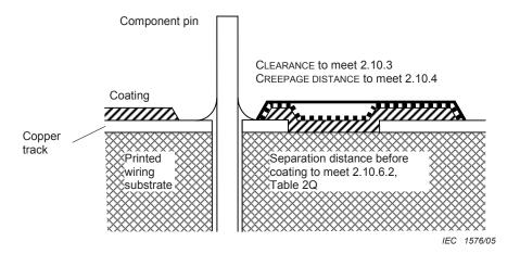
Figure F.11 - Coating over printed wiring
