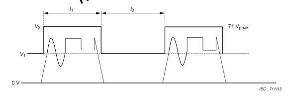
Figure 2E.2 - Voltages in SELV circuits under single fault conditions for multiple pulses above V1 (2)
