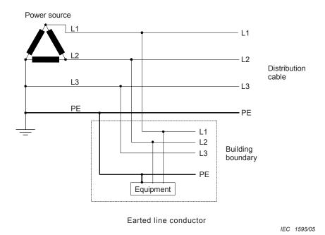
Figure V.1 - Examples of TN-S power distribution systems
