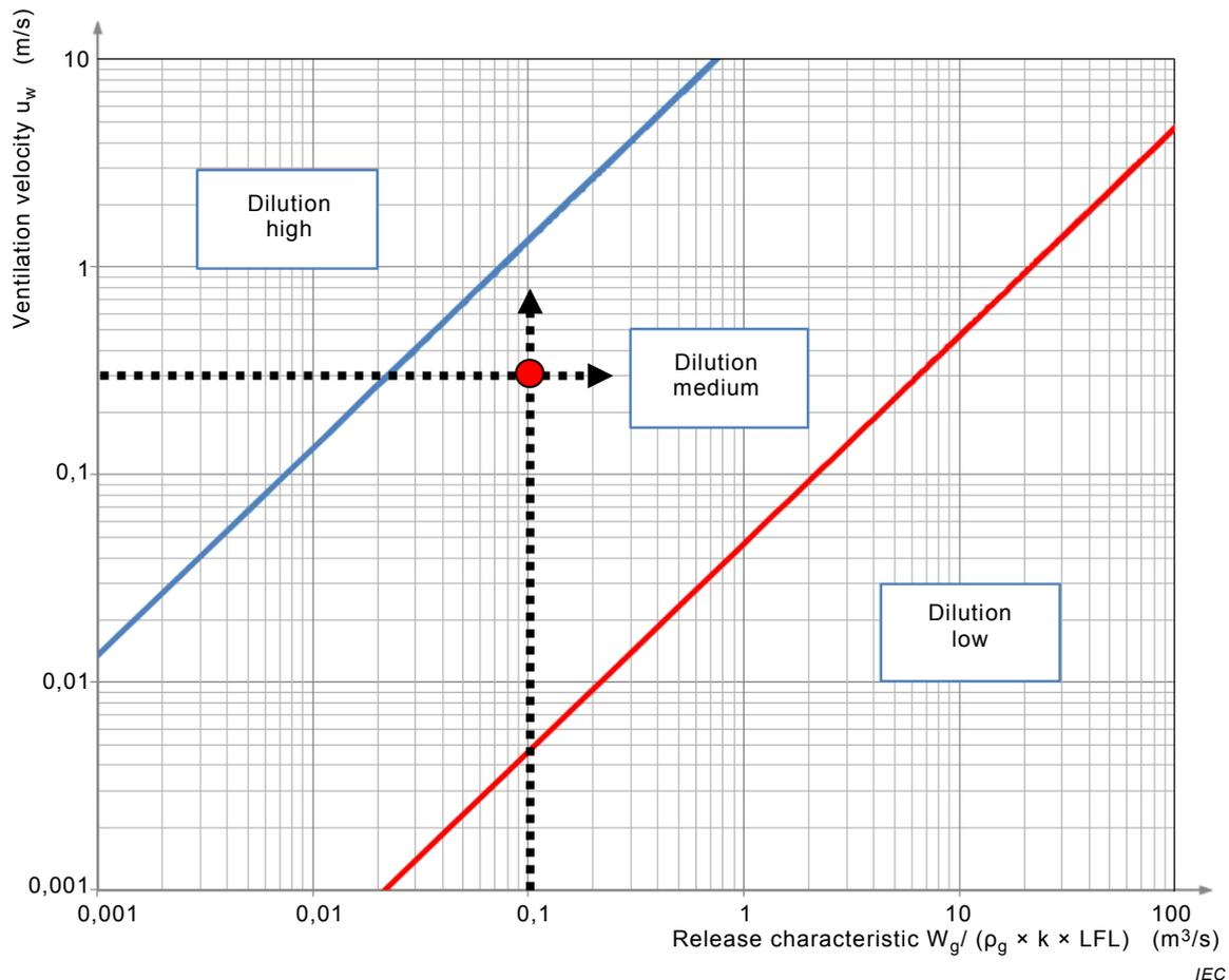
**Figure E.1 – Degree of dilution (Example No. 1)**
