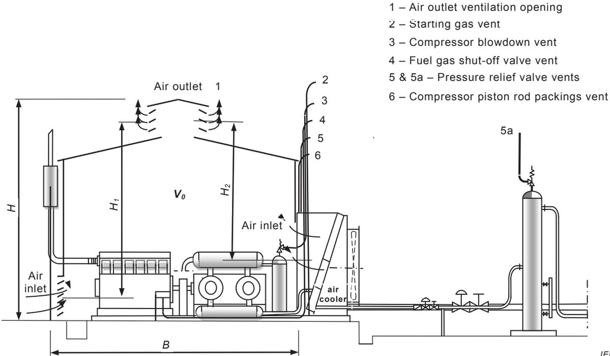
Figure E.14 – Enclosed compressor handling natural gas
