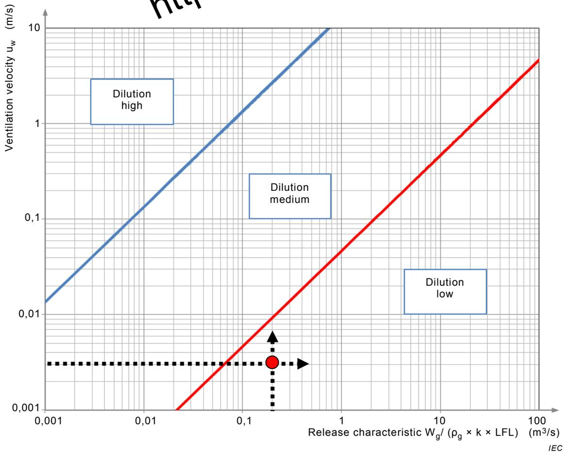
**Figure E.4 – Degree of dilution (Example No. 2)**
