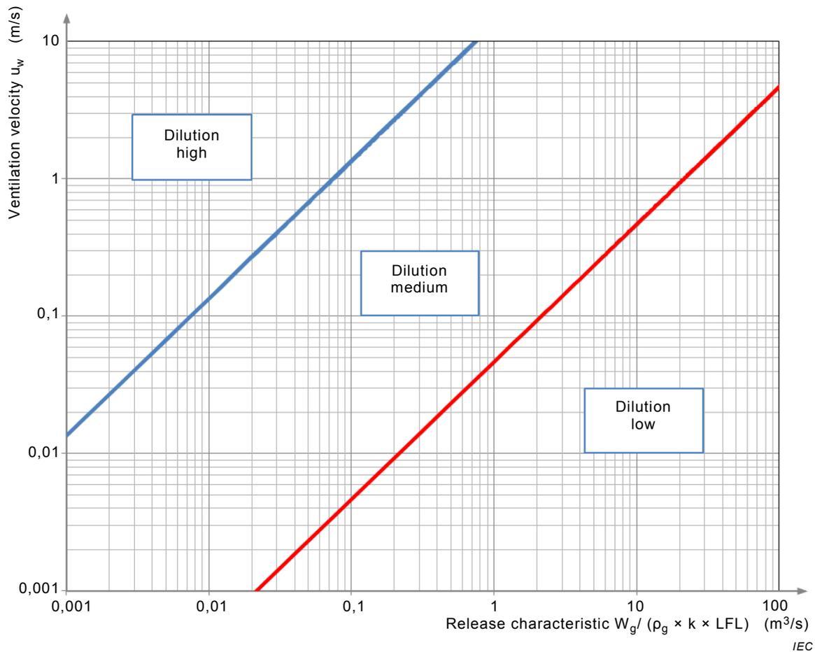
**Figure C.1 – Chart for assessing the degree of dilution**
