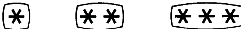
Figure 8 — Identification symbols for frozen food storage compartments (or cabinets) (for further details, see figure 17)
