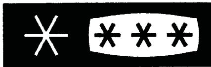
Figure 7 — Identification symbol for food freezers and food freezer compartments (for further details, see figure 16)
