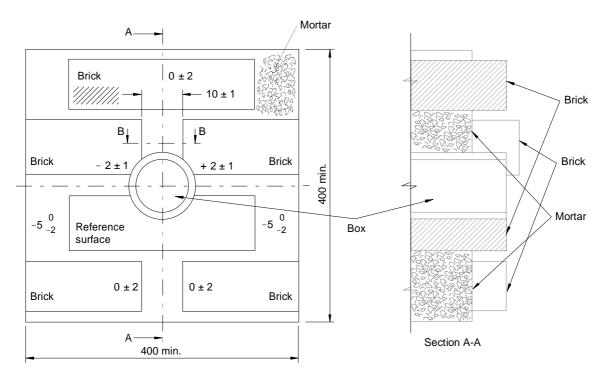
All mortar joints  $10 \pm 5$  mm thick unless otherwise specified
