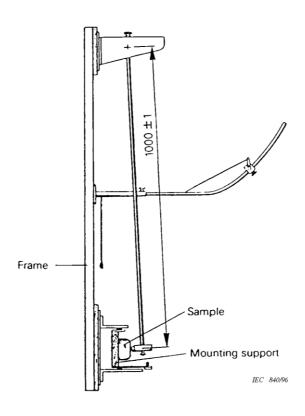
Figure 15 – Impact test apparatus
