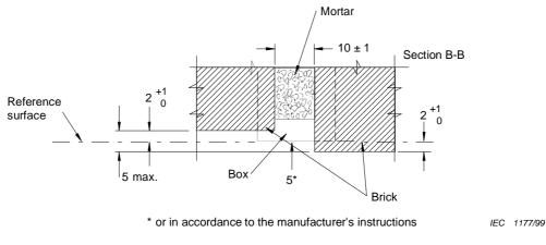
Figure 27 – Test wall in accordance with the requirements of 15.2.2
