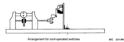
Figure 12 – Apparatus for making and breaking capacity and normal operation tests
