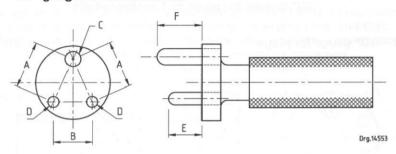
Table F.2 (a) — Dimensions of maximum "GO" gauge for socket-outlets
