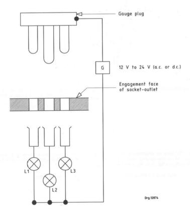
The gauge, when inserted without undue force and at any possible angle, shall cause lamp L2 to light up before either L1 or L3. When the gauge is withdrawn at any possible angle, both lamps L1 and L3 shall "go out" before lamp L2.
