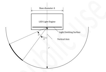
Figure 4-1: Luminous intensity distribution
