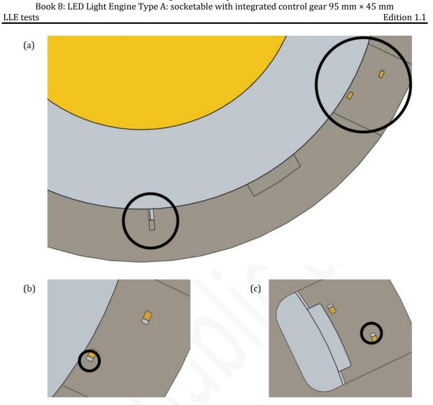
Figure 9-9: Examples of (a) test #4(a) pass, top view; (b) fail, top view; and (c) fail, bottom view
