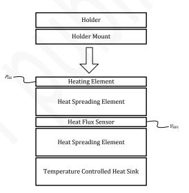
Figure 8-12: TPTF-PHJ85d-x—heat flux measurement system (illustration)
